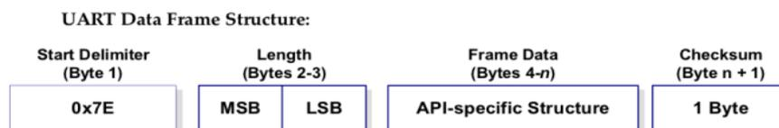
Gambar 1. Format Frame Data Mode API
