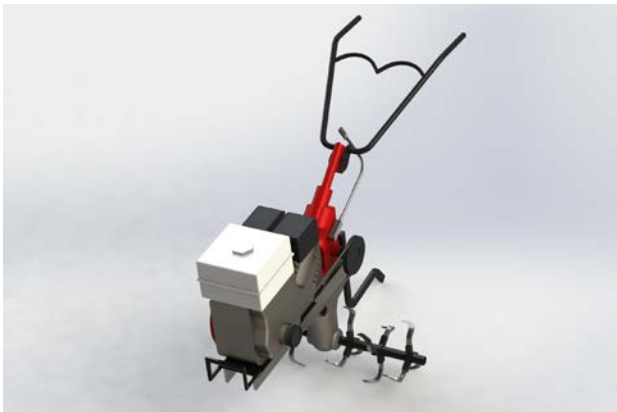
Gambar 1: Konsep Foldable Hand Tractor
