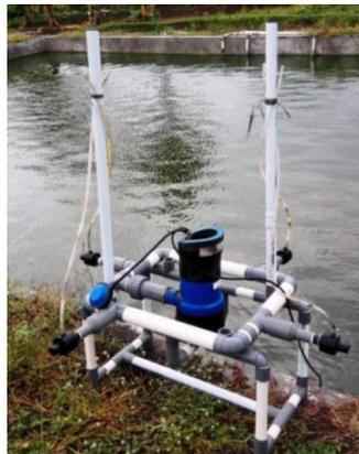
Gambar 3. Microbubble Generator
