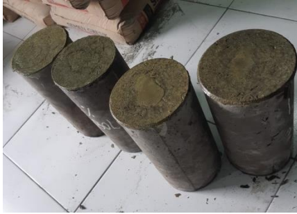
Figure 3. Cylindrical test object with coconut fiber (SSK) (Source: Preliminary analysis, 2021)
