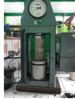
Figure 4. Concrete compressive test. (Source: Preliminary analysis, 2021)
