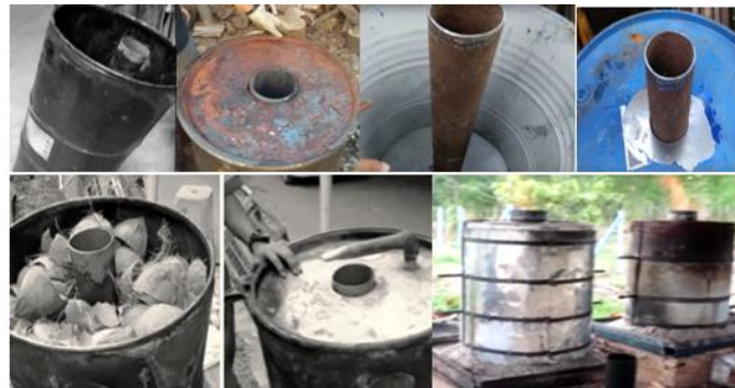
Figure 4. Drum design for making charcoal from coconut shells.
