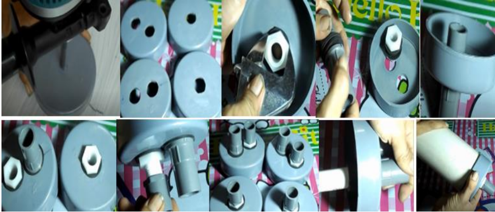
Figure 3. The process of making water filters from PVC pipes.
