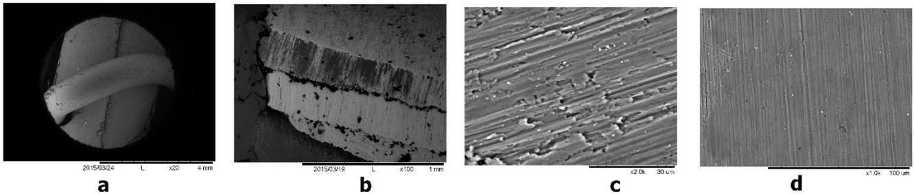
**Figure 2. (a) Copper (Cu) wire as a binder for Al plate; (b) Compressed plate piles; (c) Structure of AA1070 as a result ARB compression result; (d) Structure of AA7075 as a result of ARB compression.**
