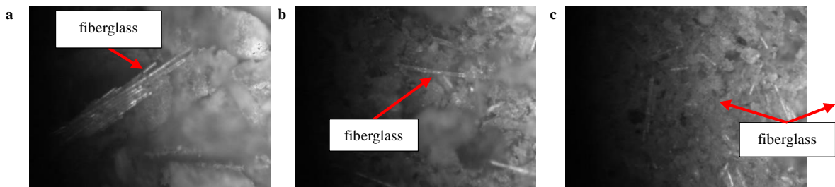
Figure 1. The findings of the PCB microscopy analysis (a) size -70+100# (b) size 100+120# (c) size -120+140# (zoom 10x).
