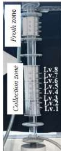
Figure 9. The levels of sensor for monitoring column flotation
