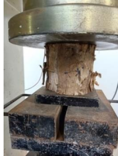
Figure 4. Compressive Strength Test of Galam Wood with 10 cm Diameter.
