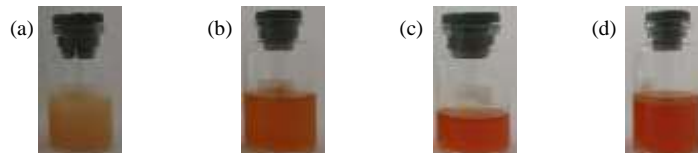
Figure 2. Soybean oil with ethanol (a) 1:4 1 hour; (b) 1:4 2 hours; (c) 2:4 1 hour; (d) 2:4 2 hours
