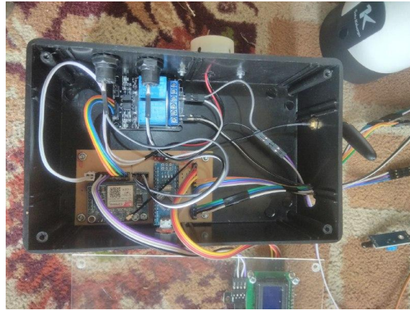
Figure 5. The prototype of a fire detection and extinguisher device using arduino nano microcontroller
