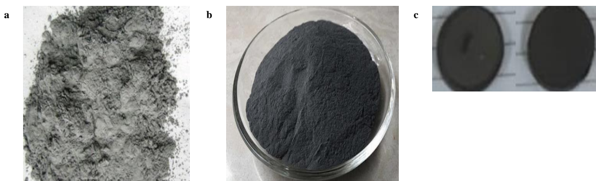
Gambar 1. -(a) Serbuk aluminium; (b) Serbuk titanium; (c) Pelet campuran Al-Ti.
