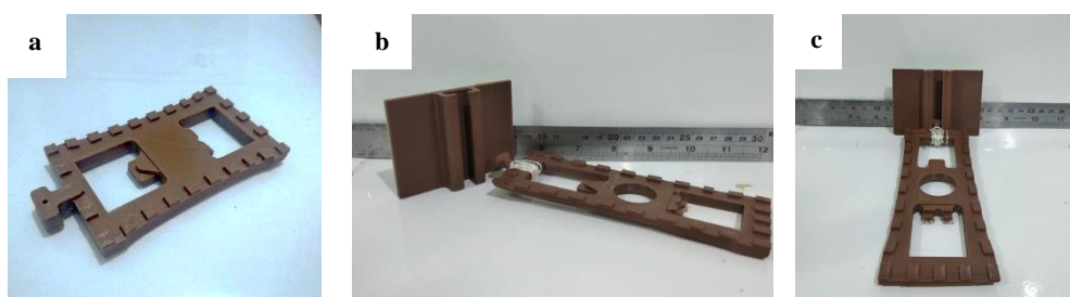
Figure 4. Printing result of the pedal design: a) Short pedal without hinge (Design B), b) and c) Long pedal with hinges (Design C)
