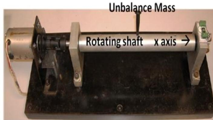
Figure 1. Vibration monitoring device in [12].
