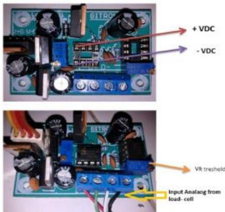
Gambar 10 . Load-cell amplifier
