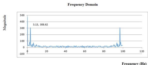
Figure 21. Analysis of vibration testing at 100 RPM with loading.
