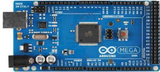
Figure 12. Arduino Atmega 2560 microcontroller.
