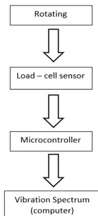
Figure 4. System block diagram
