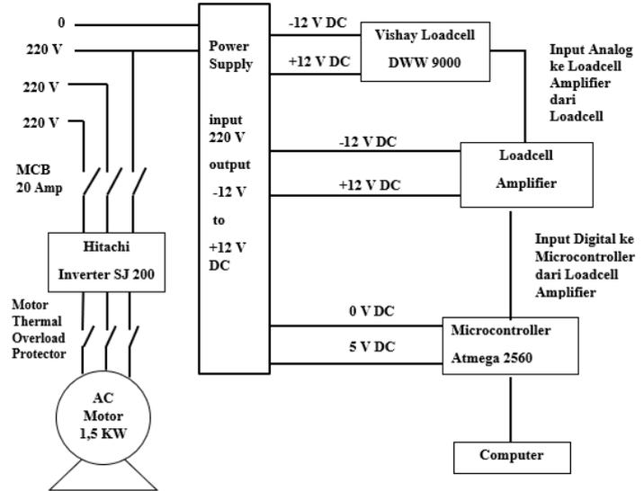
Figure 7. Wiring diagram
