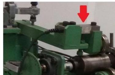
Figure 9. Load-cell position in vibration monitoring device
