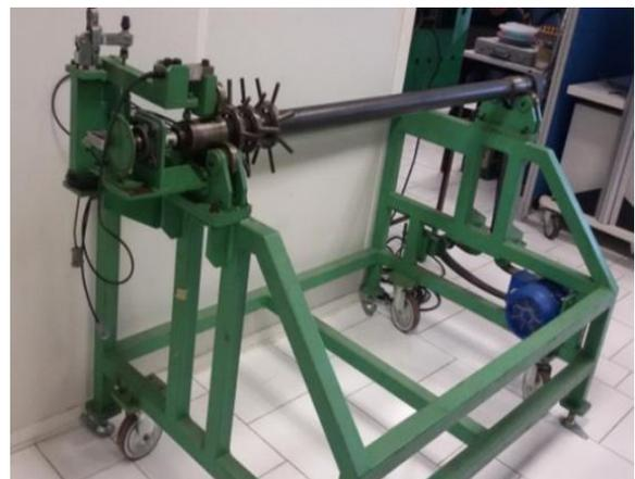
Figure 5. Prototype of vibration monitoring device
