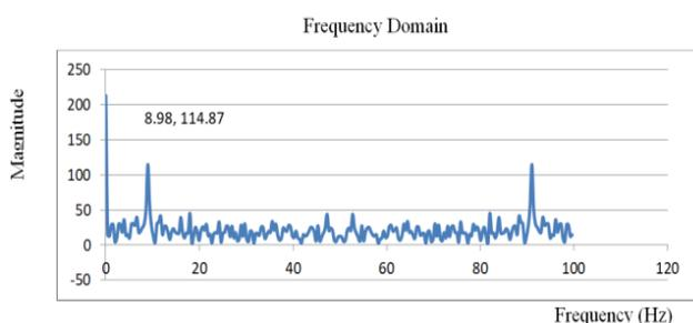
Figure 22. Vibration test analysis at 300 RPM without loading.
