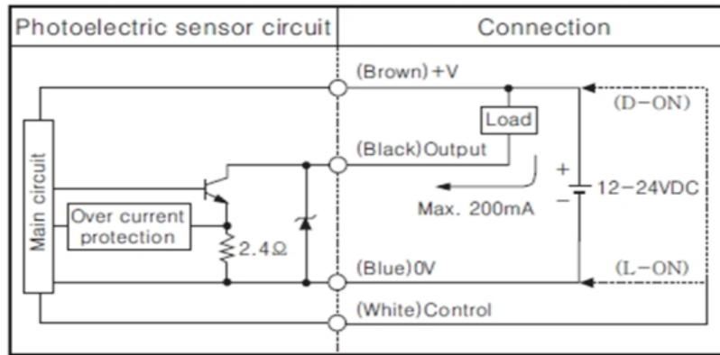
Figure 17. BUD – 30S control output diagram
