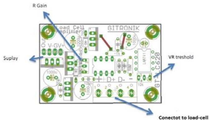
Figure 11. Load-cell amplifier schematic
