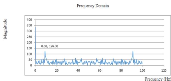
Figure 23. Vibration test analysis at 300 RPM with loading.
