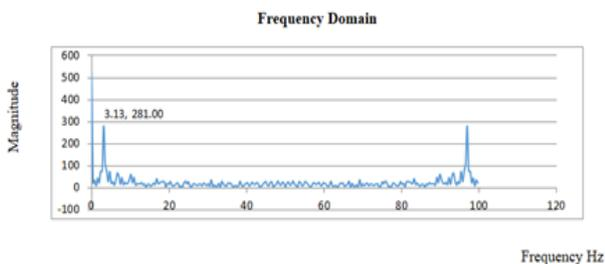
Figure 20. Vibration test analysis at 100 RPM without loading
