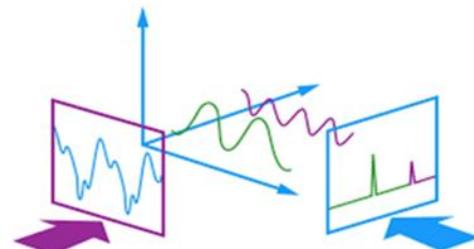
Figure 3. Signal change from time domain to frequency domain
