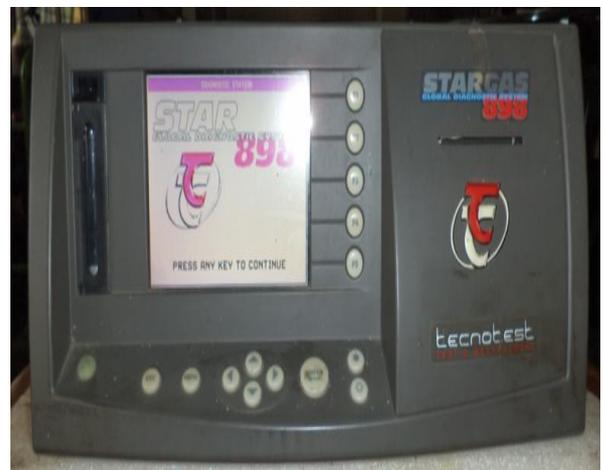
Gambar 2 gas analyzer tecnotest stargas 898
