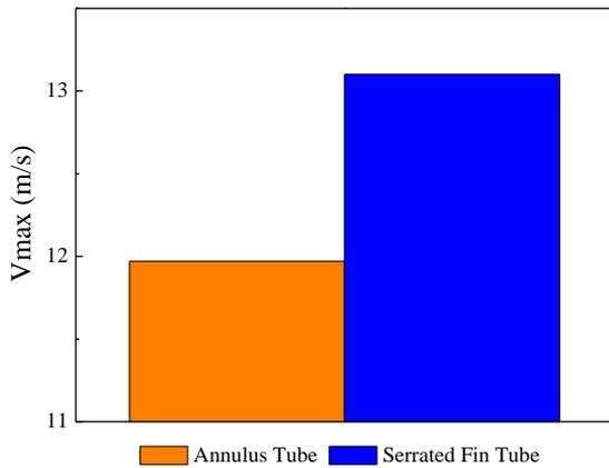
**Figure 9.**  $V_{max}$  Comparison Chart for Annulus and Serrated Fin Tube
