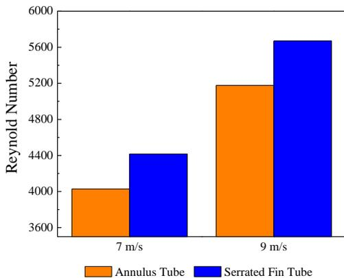
Figure 12. Reynold Number Comparison Chart for Annulus and Serrated Fin Tube at 7 m/s and 9 m/s Velocity.
