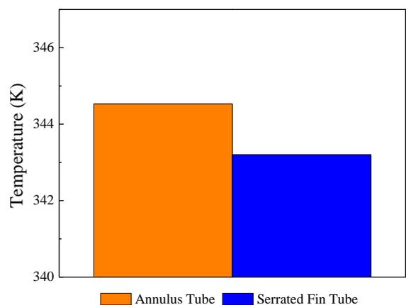
**Figure 11.** Temperature Comparison Chart for Annulus and Serrated Fin Tube.
