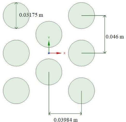
Figure 4. Design of Annulus Tube
