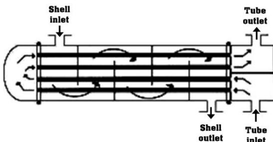
Figure 1. Shell and Tube Heat Exchanger [1].
