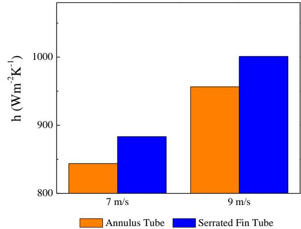
Figure 15. Comparison of Convection Heat Transfer Coefficients for Annulus and Serrated Fin Tube at Velocity 7 m/s and 9 m/s.
