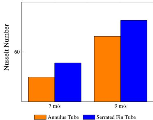
Figure 13. *Nu* Comparison Chart for Annulus and Serrated Fin Tube at 7 m/s and 9 m/s Velocity
