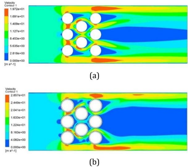
**Figure 8.** Comparison of Velocity Distribution (a) Annulus and (b) Serrated Fin Tube
