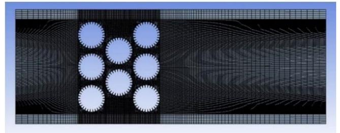
Figure 7. Meshing Serrated Fin Tube
