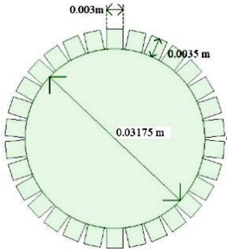
Figure 5. Design of Serrated Tube
