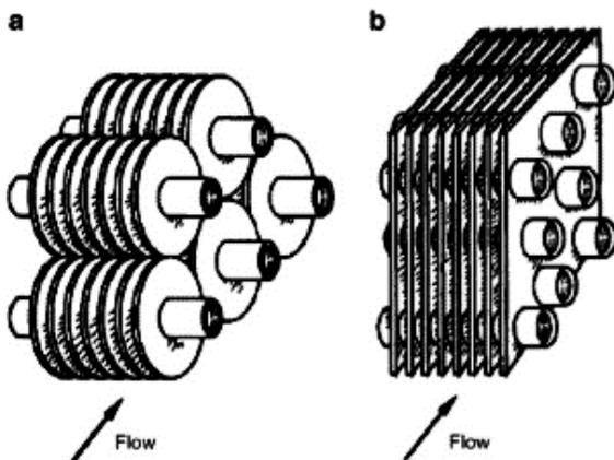
Figure 3. Fin Tube Exchanger Configuration. (a) Individually Fnned Tubes. (b) Flat Fin with Continuous Form On an Array of Tubes [5]
