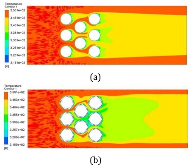
**Figure 10.** Comparison of Temperature Distribution (a) Annulus and (b) Serrated Fin Tube.
