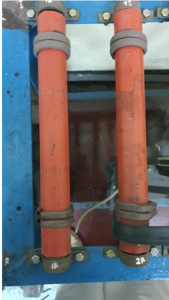
Figure 6. Rubber seal for slip prevention.
