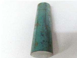
**Gambar 4. Material benda kerja Baja Aisi 1045**
