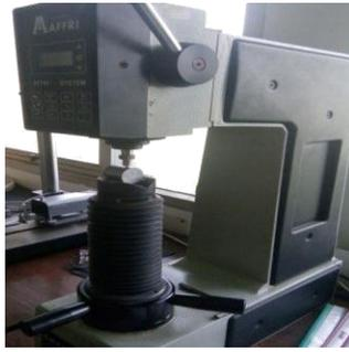
**Gambar 2. Alat uji kekerasan HB 30 tester**
