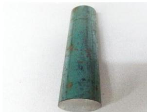
**Gambar 4. Material benda kerja Baja Aisi 1045**
