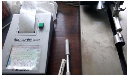
**Gambar 3. Alat Uji Kekasaran Surface Roughness Teste**
