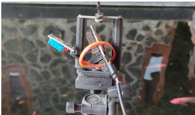
Figure 8. DHT11 sensor is placed openly on the edge of the fish pond.
