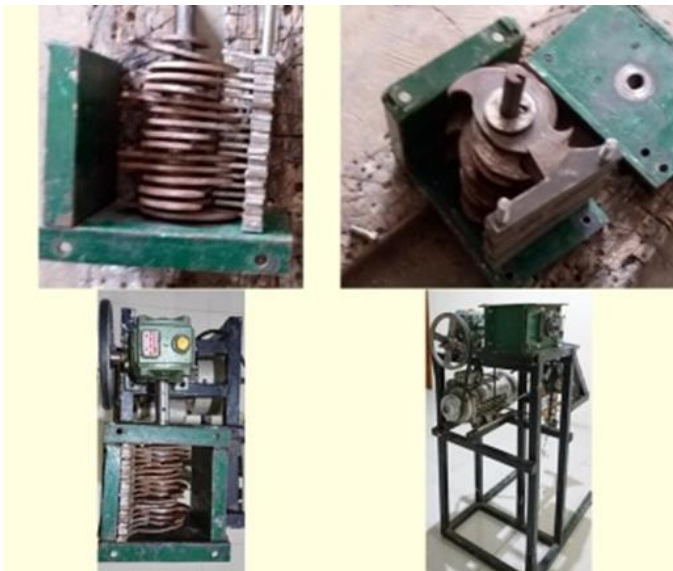
Figure 8. Assembly of cutting edge in the shredder plastic machine
