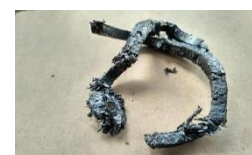
Figure 5. The remaining use of non-OEM packing with wire fibers
