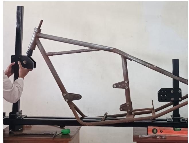
Figure 6. Application of the universal jig with chopper frame
