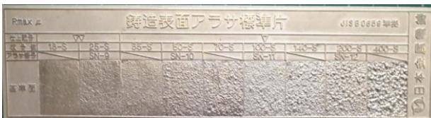
Gambar 6. Standard Roughness Test JIS B -0659.
