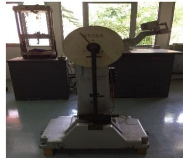
**Gambar 5.** Mesin uji impact *charpy*.
