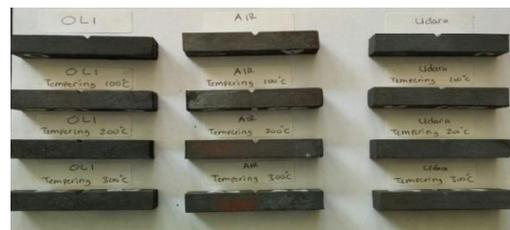
**Gambar 6.** Sampel uji impact *charpy*.
