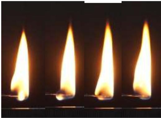
**Gambar 6.** Visualisasi microexplosion biodiesel
