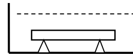
Figure 2. The specimen stand alone in the electrolyte. The support at ends are intended to prevent the effect of aeration differential cell at the bottom.
