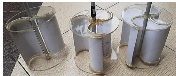
Figure 5. Savonius Hydro Turbine: (a) two blades; (b) three blades; (c) four blades
