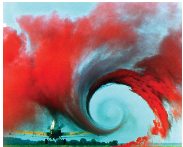
Figure 1. Wing-tip vortex visualized by smoke.
