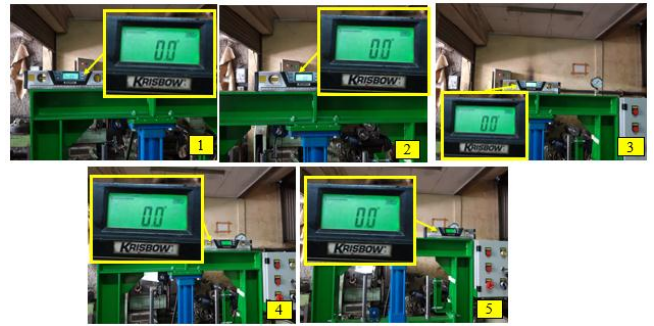
Figure 7. Measurement of datum A with a waterpass
