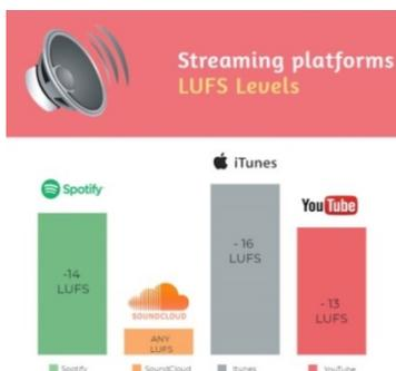
**Gambar 4.4 Streaming Platform LUFS Levels**
