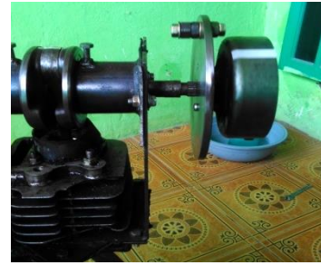
Figure 5. modification of the flywheel on the Stirling engine
