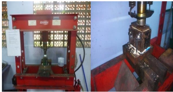
Figure 2. Particleboard composite compaction process
