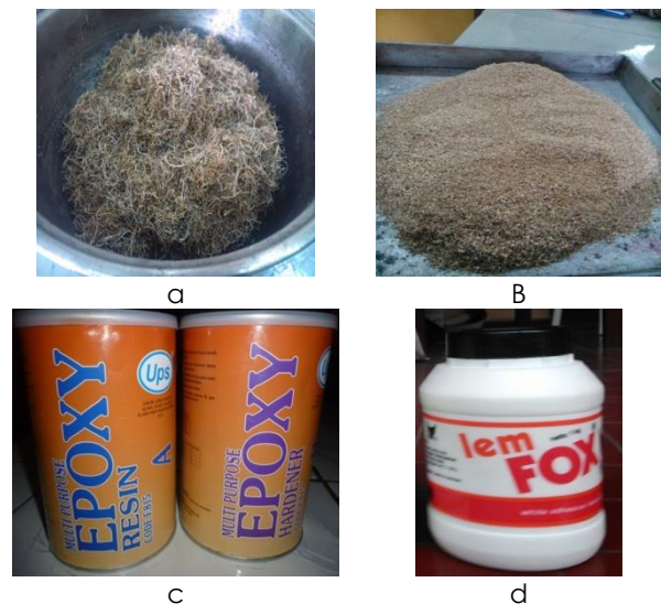
Figure 1. The constituent materials of particle board composites
