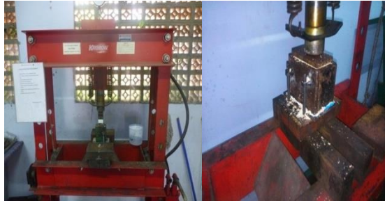
Figure 2. Particleboard composite compaction process
