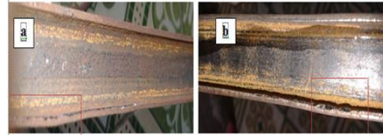
(a). Wings are not Perfectly Bent. (b). Material Damage.
