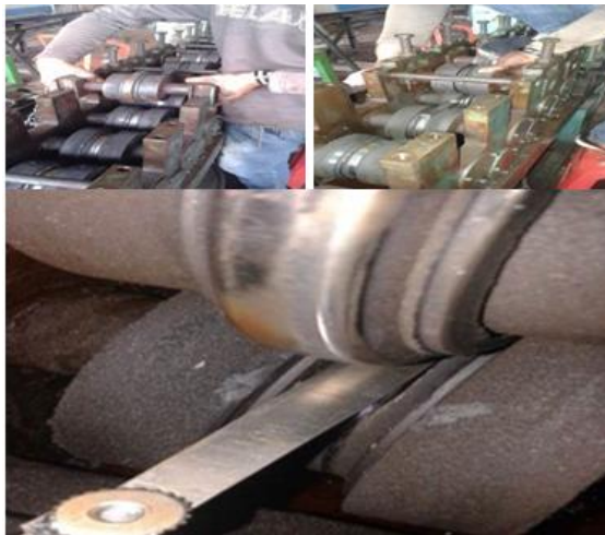
Figure 6 Measurement of Roll Gap
