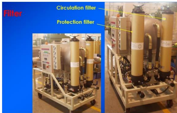
Figure 12. Circulation Filter and Protection Filter
