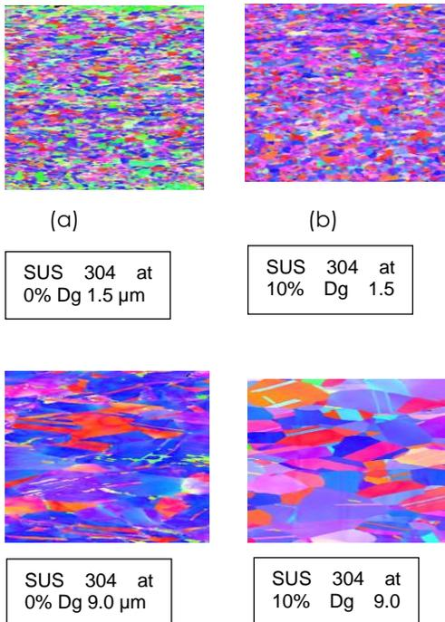
**Figure 4.** Specimen ASS SUS 304 TMF of Grain Deformation
