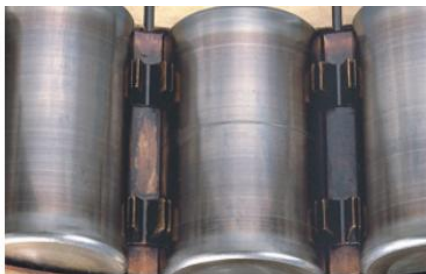
Figure. 2 Scratches on the surface of the rolling elements
