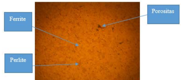
Figure 2. AISI 1020 low carbon steel specimen 100x magnification
