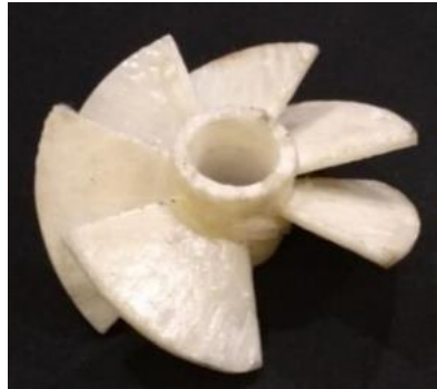
Figure 1. Blade failure due to axial load (Darsono et al. , 2021)
