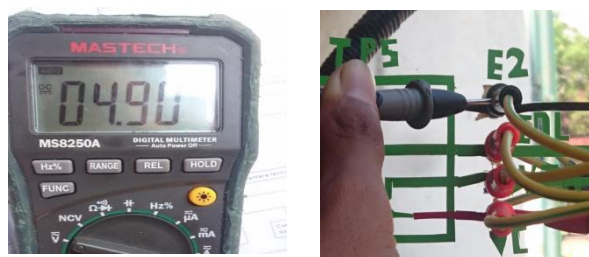
Figure 2. TPS voltage check at terminal VC-E2
