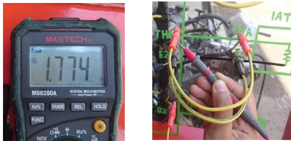
Figure 7. Checking the intake air temperature sensor voltage
