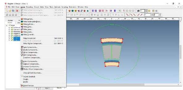
**Figure 7.** Make simple coil
