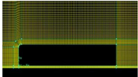
Fig 5. Meshing bluff body without adding Diffuser
