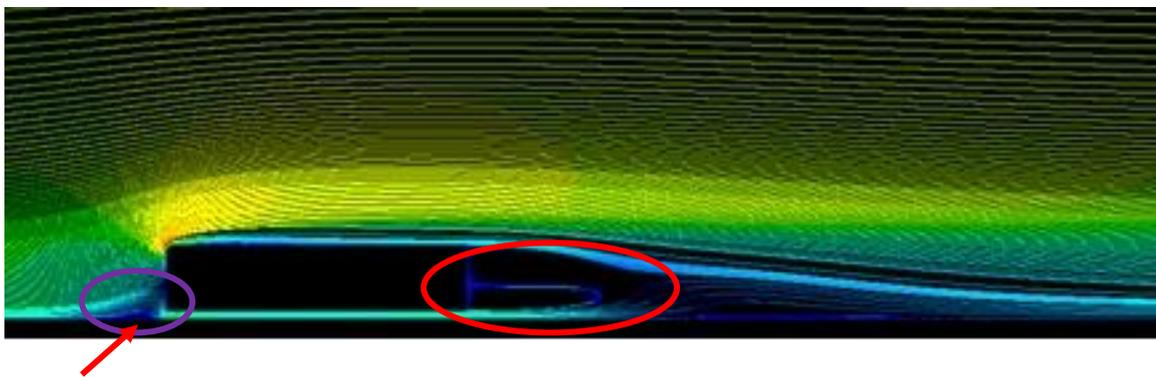
Fig 7. Pathline Velocity Model Bluff body Without Additional Diffuser
