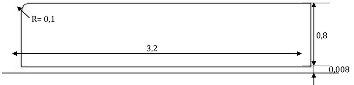
Fig 3. Bluff body Without Additional Diffuser
