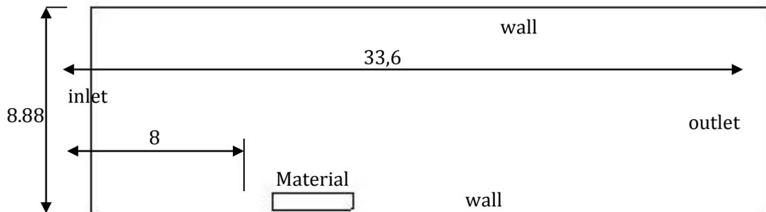
Fig 1. Dimensions and boundary conditions of numerical simulations
