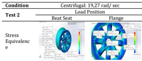
**Table 6.** Tensile of test load simulation results in 3
