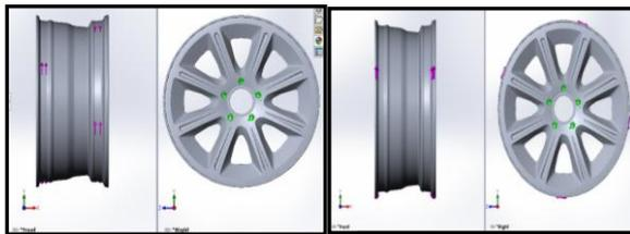
Figure 6. Boundary condition by giving fixed support and giving equivalent force to the seat and flange beat
