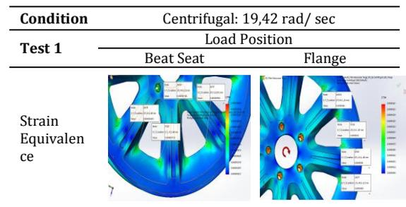
**Table 9.** The strain of the test loading simulation results in 2
