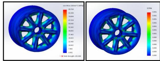
Figure 7. (a) tension and (b) strain that occurs on the seat beat and wheel flange due to bending moment
