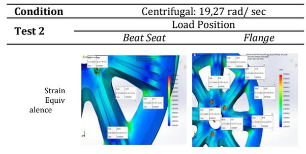
**Table 10.** The strain of the test loading simulation results in 3
