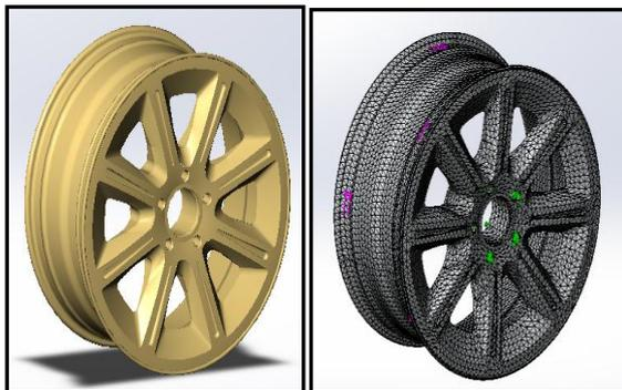
**Figure 4.** Geometry and meshing models remodeling results
