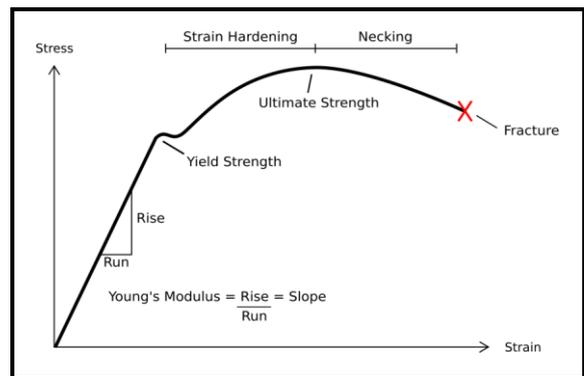
**Figure 5.** Stress Curve - Strain Diagram
