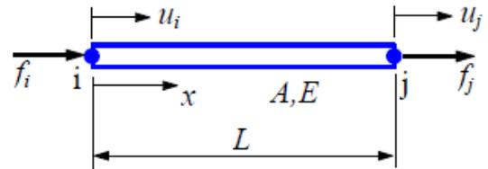
**Figure 2.** Free body bar diagram
