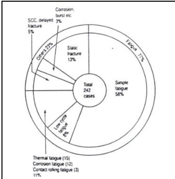
**Figure 1.** Distribution Mode Failure
