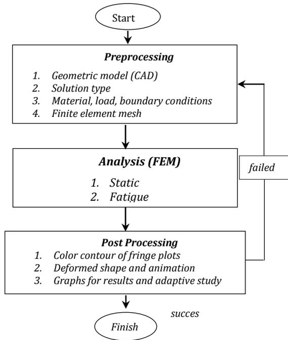
**Figure 3.** SolidWork simulation flowchart
