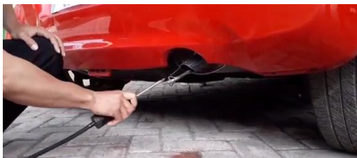
Figure 3. Technique of Exhaust Emission Testing Sources: Wraiter (2017)
