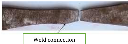
Fig 8. Friction test tensile material with E 7016 electrode
