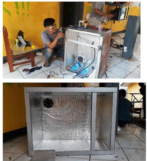
Figure 3. Initial stage of dryer machine manufacturing
