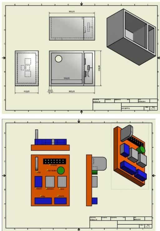
Figure 2. Electrical Dryer Machine Design
