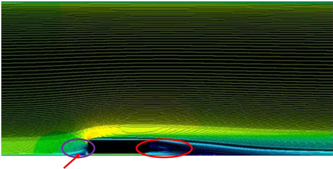
Fig 6. Pathline Velocity Model Bluff body with Additional Diffuser
