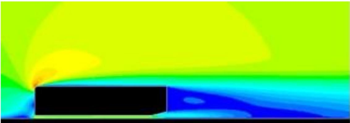
Fig 8. Contour Velocity On Bluff Body Model With Diffuser Addition
