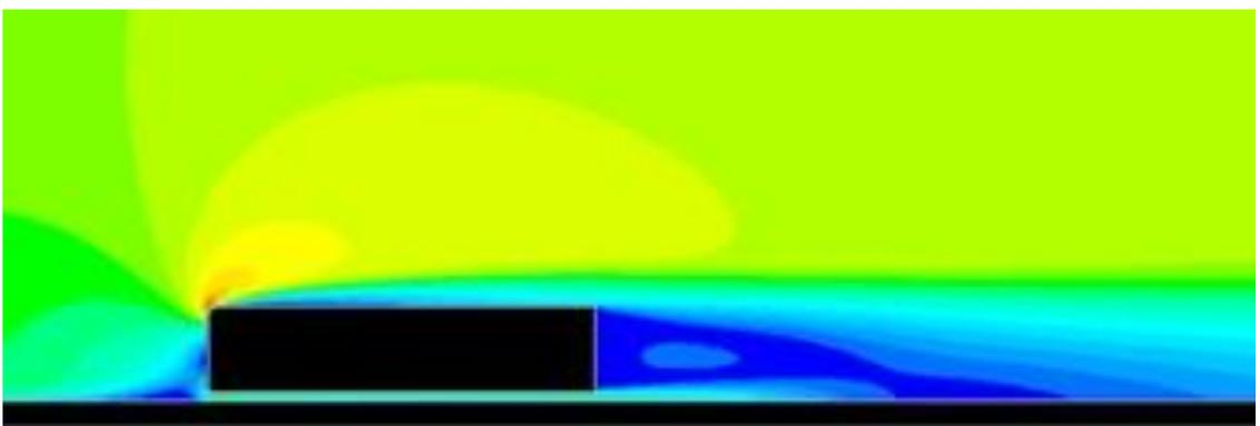
Fig 9. Contour Velocity In Bluff Body Model Without Diffuser Addition
